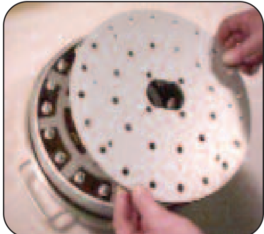
Figure 7: Now lift the Plug Plate, exposing the Divider Assembly.
