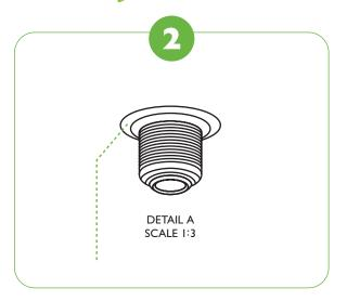
Add 1/4" String of Plumber's Putty to Underside of Drain Grid and press firmly around drain face. Place Drain Grid into bottom of Bowl and press firmly to seal against Bowl.
