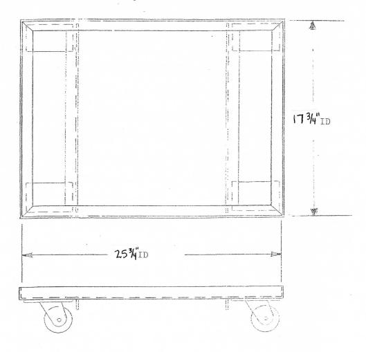
This dolly is made from 1-1/4" X 1-1/4" angle and has four 3" swivel polyolefin casters and painted blue
