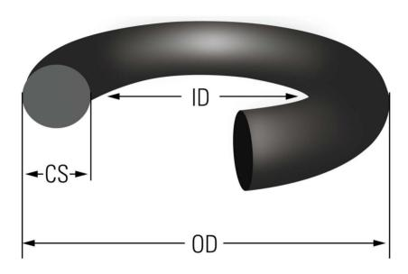
Colors of the replacement o-rings may not correlate to your machines accessories o-ring. Please confirm size of the o-ring when replacing.
