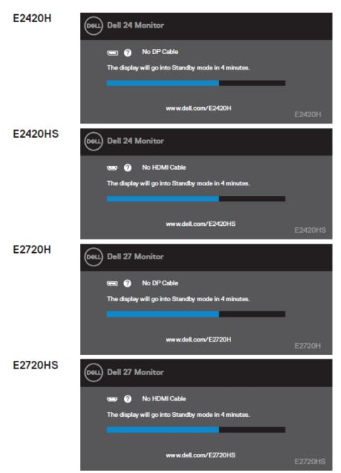
NOTE: This box also appears during normal operation, when the video cable is disconnected or damaged.
