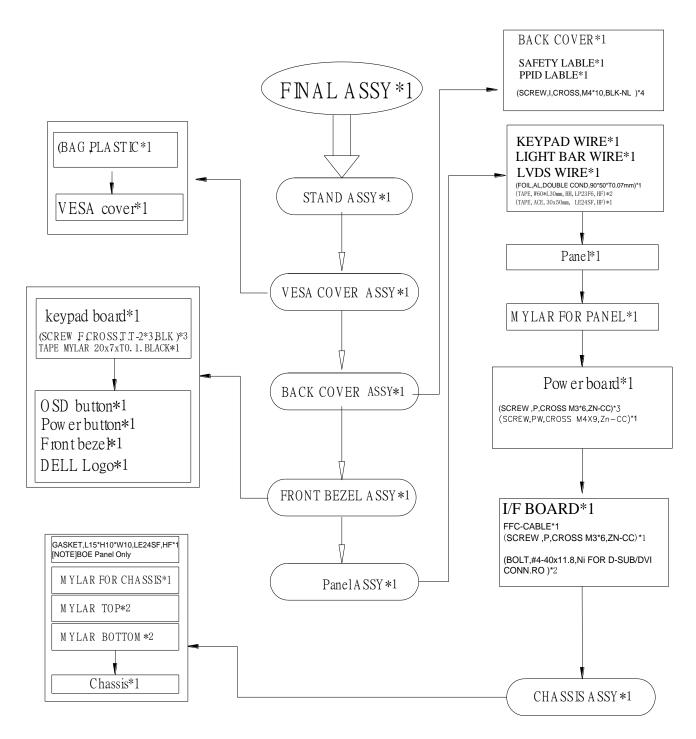
Note: 1. The arrows point out the direction of disassembly. **Disassemble the slot of Back cover from monitor**
