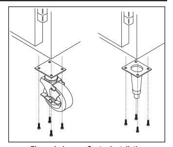
Figure 1. Leg or Caster Installation
