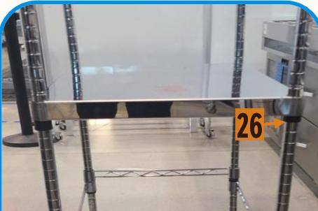
**B** Install the solid surface shelf designated for pizza peel storage at Slot #26.
