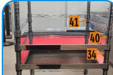
**C** Install the solid surface shelf designated for bottle storage at Slot #34. Install two 24-inch hanger rails at Slot #40 and one 18-inch hanger rail at Slot #41.
