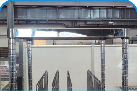
**F** Install a solid shelf at the top of the unit to act as a cover. This will prevent dust and debris from heating vents from coming into contact with food containers.
