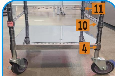
**A** Using a rubber mallet, insert all four casters securely into the base of each pole. Position a solid shelf for pan storage at Slot #4. Install two 24-inch hanger rails at Slot #10 and one 18-inch hanger rail at Slot #11.
