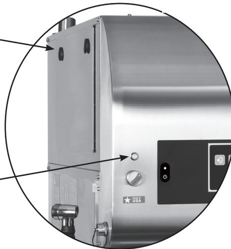
**Timed Latching Mechanism:** In order to evacuate steam and grease-laden air from the oven interior, this mechanism prevents the operator from fully opening the oven door for 20 seconds. Longer wait times can be programmed into the control. The mechanism automatically disengages at the end of a pre-set time allowing full door extension.
