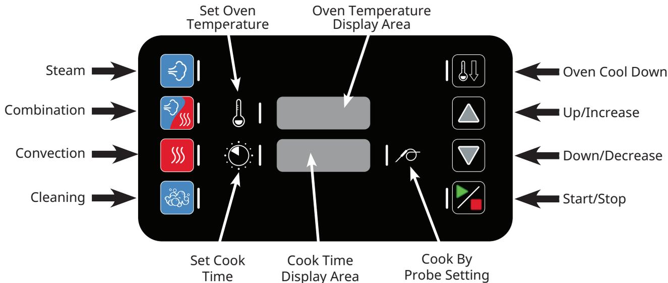
The Steam mode provides the operator with the ability to steam, poach, or blanch. This mode will automatically steam at the boiling point of water; quick-steam above the boiling point for faster cooking results; or low temperature steam, below the boiling point, for more delicate products such as pâté, mousse, seafood, or custard.
