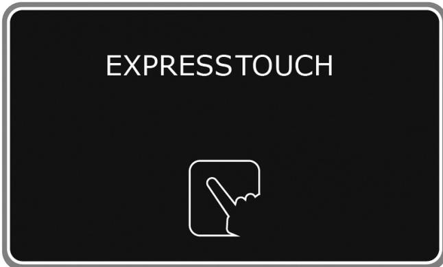
When the oven is powered on, the ExpressTouch screen illuminates. "Loading" indicates that the software is booting up. The screen will also indicate what level of progress has been made as the software becomes fully operational.
