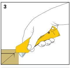
**AFTER CUT**, the guard will automatically cover blade and **LOCK** again.
