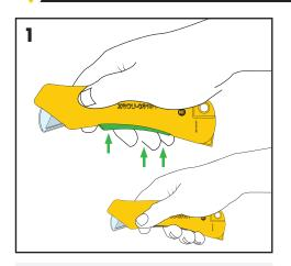
**SQUEEZE** and hold trigger. This unlocks the guard.
