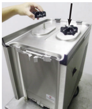
Install mixing impeller.
