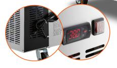
Equipped with a back right 115V electrical connection, 1/6 hp compressor, and R290 refrigerant to cool the cabinet and electronic temperature controls.
