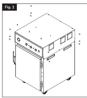
1. Remove all (15) screws as shown on the top, right, and left sides of the bottom unit. (Fig. 1)
