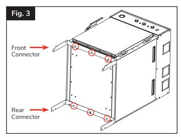
3. Install (2) brackets to bottom of the cabinet that 4. Place the upper cabinet on top of the lower will stack on top with (6) screws. (Fig. 3) NOTE: Pay attention to the direction of the bracket.
