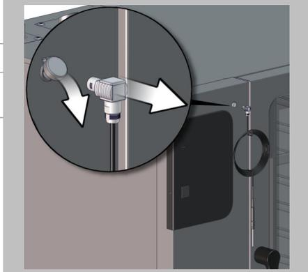
Unplug the external core temperature probe or sous vide probe from the unit case.
