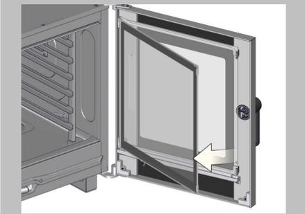
3. Carefully swing the inner pane out of its mount.
