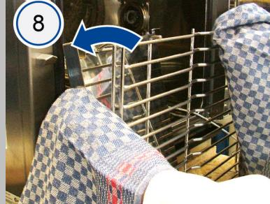
Swing the air distributor backwards (8) and disconnect the rack from the air distributor.
