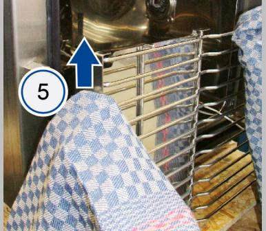
Push the air distributor upwards (5).
