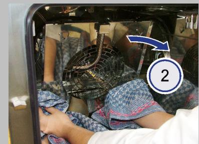
Push the suction panel upwards and remove it (2).
