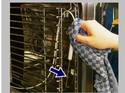
Slide the core temperature probe into the holder.
