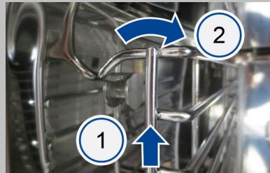
Slightly lift the rack at the front (1) and then lift it over the front holder (2).
