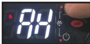
3. Press and **RELEASE** the “SET” button. The current alarm setting will be shown.
