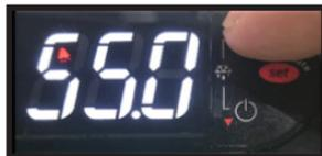
5. Press and **HOLD** the “SET” button for 5 seconds to confirm and save the new value. When complete, the current temperature will be displayed. **RELEASE** the “SET” button.
