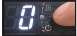
3. Press the "UP" button until "22" appears. This is the password. **RELEASE** the "UP" button.
