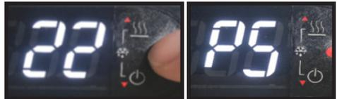
5. When you get to the parameter you want to change press and **RELEASE** the "SET" button. The current setting will be shown in the display. Use the "UP" or "DOWN" button to change the value. Press and **HOLD** the "SET" button for 5 seconds to confirm and save the new value. When complete, the current temperature will be displayed. **RELEASE** the "SET" button.
