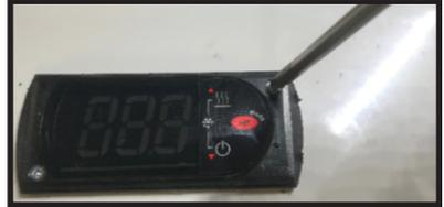
**Plastic Keeper.** When turning screw counter clockwise, this will rotate this keeper.
