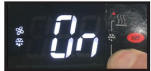
2. To turn controller back ON, press and HOLD the “POWER/DOWN” button for 5 seconds. Controller will resume normal operation.
