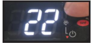
4. Press and **RELEASE** the "SET" button. "PS" will appear in the display. You now have access to the tech service level parameters. Use the "UP" or "DOWN" button to navigate to the required parameter.
