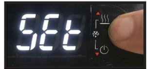
2. Press the “UP” or “DOWN” button to adjust to the new set-point value. Here the “UP” button was pressed to change the set-point from 36°F to 37°F.
