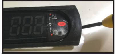
3. Use a PZ1 screw driver (#1 Phillips will also work) and turn both screws ¼ turn counter clockwise. This will rotate the plastic keeper behind the sheet metal to be able to pull out the electronic control.
