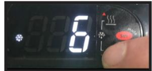
5. Press and **HOLD** the “SET” button to lock in this new value. When the display returns back to cabinet temperature, **RELEASE** the “SET” button.
