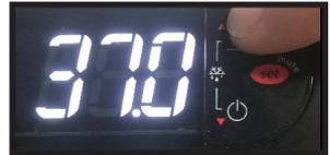
3. Press and **RELEASE** the “SET” button to lock in the new set-point. The control will now resume normal operation with the new set-point.
