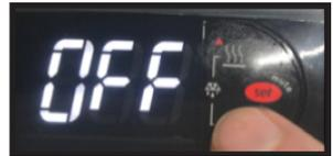
When the control is powered “OFF”, OFF will alternate in the display with the current appliance temperature.
