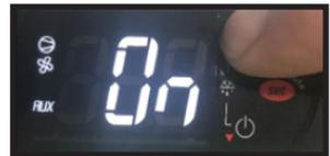
2. To change the current state of the AUX Heaters, press and **HOLD** the AUX HTR button. The display will show the current state of heater operation. After 5 seconds, the heater will switch to the opposite state and the display will return to displaying the cabinet temperature. **RELEASE** the button.
