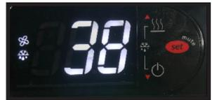
**Defrost will terminate when the pre programmed temperature or time duration has been reached. The manual defrost can also be manually terminated by pressing and holding the “Up” and “Down” button for 5 seconds.**
