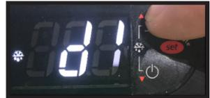
3. Press and **RELEASE** the “SET” button. The current defrost interval will appear in the display.
