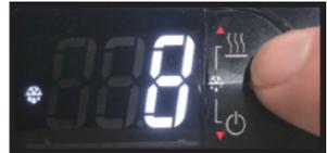
4. Press the “UP” or “DOWN” button to adjust to the new defrost interval. Here the “DOWN” button was pressed to change the interval from every 8 hours to every 6 hours.
