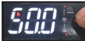
4. Press the “UP” or “DOWN” to get to the new alarm set-point. Release the button. In this case the “UP” button was pressed until the new set point of 55.0°F was reached.
