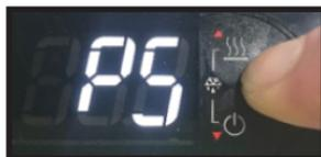
2. Press the “UP” button until “AL” (Low Alarm Setting) or “AH” (High Alarm Setting) appears in the display. **RELEASE** the “UP” button.
