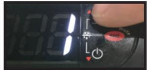
5. Press and **HOLD** the “SET” button for 5 seconds to confirm and save the new value. When complete, the current temperature will be displayed. **RELEASE** the “SET” button.
