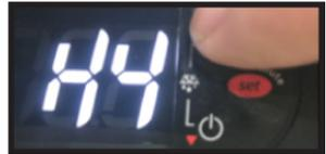
3. Press and **RELEASE** the “SET” button. “0” will appear in the display. 0: alarm beeper active.
