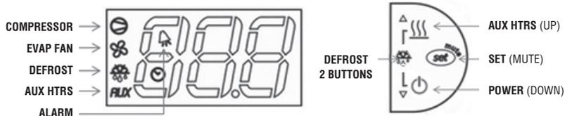
The control icons shown above will be illuminated when the associated function is active. If the icons are flashing, it means the function will be activated after the controller delays are finished.
