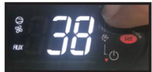
The control has a built in energy saving feature for the aux (anti-condensate heaters). When in the ON position, the "AUX" icon may not illuminate indicating the AUX heaters are not currently energized. The control will automatically energize the AUX heaters when the conditions require these heaters to be activated.
