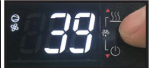
**For example:** If a sensing device in the cabinet reads 38° and control display shows 41°, follow steps above and decrease current offset value by 3 (if current offset value was 0, change to: -3.0 and save.)
