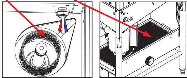
2. The drain stopper is installed.
