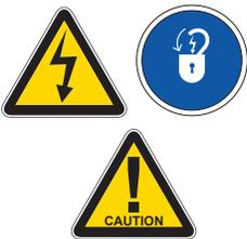
**CAUTION!** Heater contactor wires must NOT be connected before water fills machine the first time!
