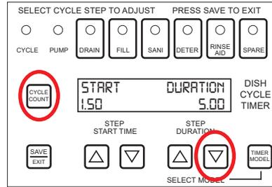
2. Resets all settings to factory defaults for the active model. Cycle count is unaffected by the reset.
