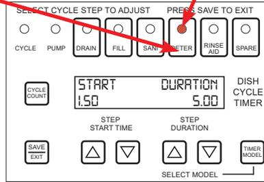
2. Change STEP START TIME or STEP DURATION using ARROW buttons (adjustments are made in 0.25-second increments).
