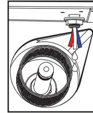
4. Detergent is dispensed during the wash cycle. The amount of detergent might need to be adjusted depending on water quality and type of detergent.
