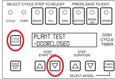
2. Press and hold the DRAIN button. The DRAIN output stays on while the button is held. The output turns off when the button is released. Repeat for the other seven buttons (use SAVE/EXIT to activate CYCLE output, use CYCLE COUNT to activate PUMP output). Second row of display shows outputs and inputs that are active.
