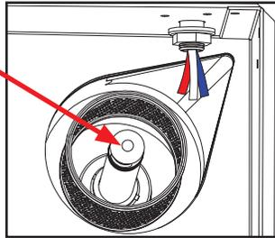
3. The wash/rinse arms (top and bottom) are installed and secure.
