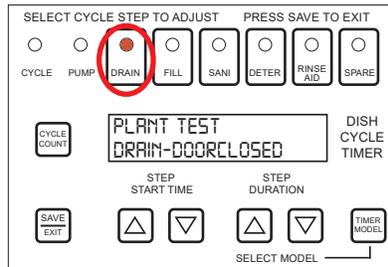
3. Plant test mode can also be used to prime chemicals if the machine has no priming function. Open door and press and hold the SANI button until sanitizer is seen entering the wash sump/tank and no air is in the line.
