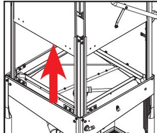
3. Remove drain stopper and allow tub to drain.
