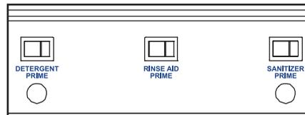
3. To prime the pumps, hold the switch in the momentary position until the chemical is seen entering the sump.
