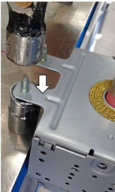
**1.** The new magnetrons come with four pressed studs for fixing. These studs need to be removed before fitting the magnetron to the oven.
