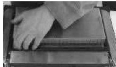
**6.** Press down firmly to tightly secure the door seal onto the door. Ensure it is level and square. Wipe off any excess sealant protruding for the door seal.
