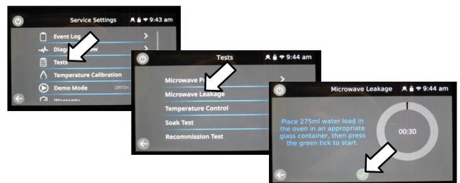
**17.** Finally, remove the bowl of water from inside the cavity and select the recommission test (if the recommission test is greyed out, it means the oven is above the desired temperature and the function is disabled). Follow the onscreen instructions and record result.
