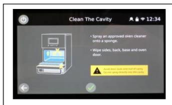
6. Spray Merrychef approved cleaner onto a sponge and wipe onto the sides of the inside of the oven, the back, the base and the oven door. Avoid the roof and door seal.
