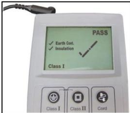
1. Connect the mains lead from the appliance to a portable appliance tester
