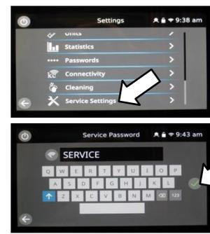
**11.** Enter the service settings, password SERVICE to access the service screen. Use the displayed oven serial number if this is invalid.
