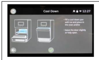
2. Place a pan of ice into the oven to speed up the cool down process or leave the door slightly open. Press the green tick to continue at each stage.
