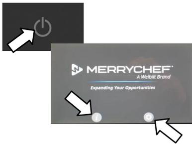
**8.** Switch the oven on and record the Serial Number. Check the firmware is correct, update if older version is observed (select the 'cog' to enter settings).
