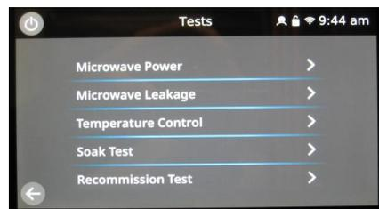
Enter Service Settings screen and select 'Tests'. For details see "Accessing the service information" section 5.1. Select the required individual test for the appliance to perform.
