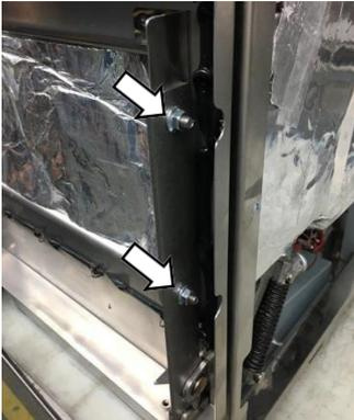
**4.** Unfasten and remove the four M5 flange locking nuts & M5 hex head bolts from the door hinges
