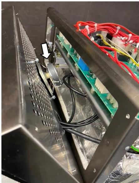
The speaker is located on the rear of the front panel, behind the UI, by two M7 hex nuts and connected directly to the UI loom.
