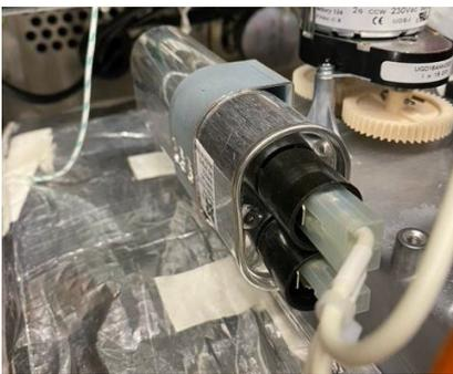
The high voltage capacitor is located on top of the cavity and is fixed by a sheet metal bracket and a pozidriv (PZ2) screw
