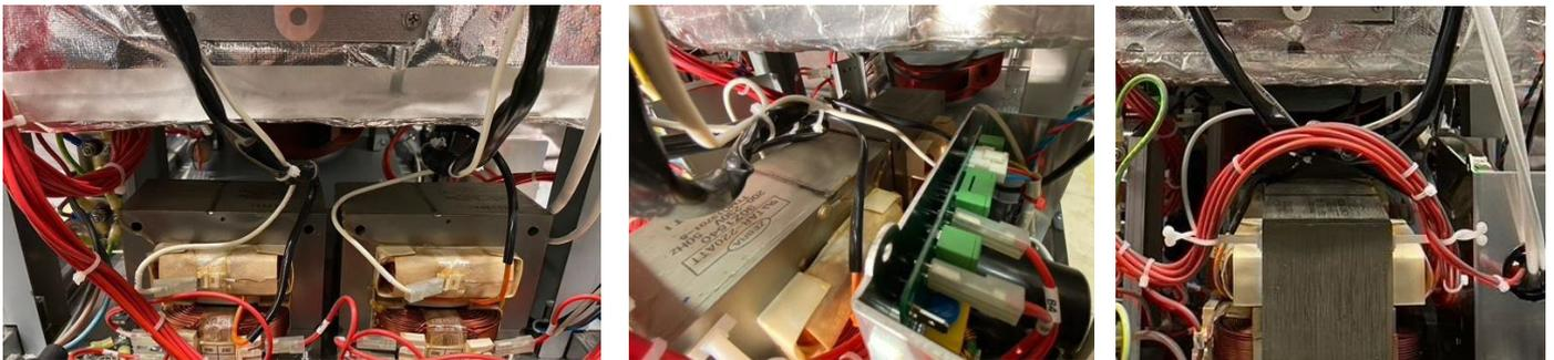
The X16 has two HV transformers, side by side, at the rear of the oven, under the cavity.
