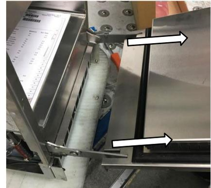
**6.** Slide door off the hinges to remove.
