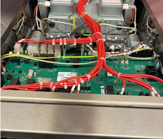
The IO Board extends over the width of the oven behind the front panel, above the cavity. It is mounted to the cavity frame.
