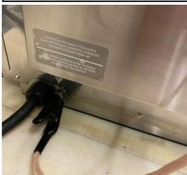
2. Connect the earth from the portable appliance tester to the equipotential bonding point on the oven.
