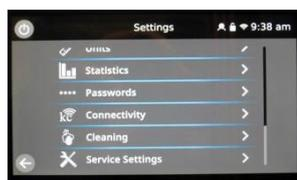
**13.** Select the oven statistics and reference the service check sheet for recommended replacements, advise the customer on actions required.
