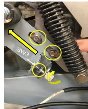
2. Loosen the interlock adjuster and locking nuts.
