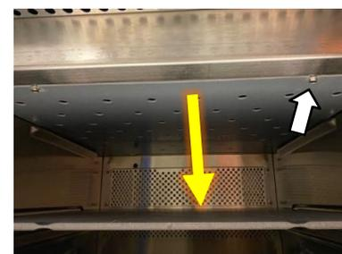
**7.** Remove & refit upper impinger plate inspecting for cleanliness and signs of damage (if required follow the instructions laid out in the replacement impinger Kit). Visually check the partition plate for signs of discolouration or damage.
