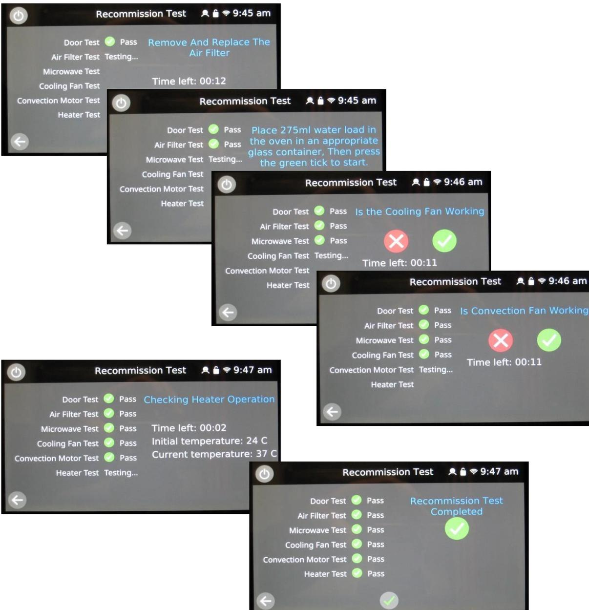
Note: If the door is opened during the microwave circuit test, the process will stop and record a failure.
