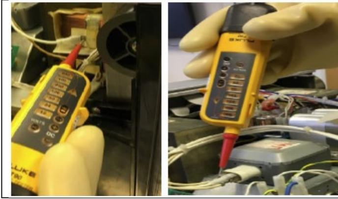
Re-test your proprietary voltage tester is working correctly and test to ensure the capacitor is discharged (dead) at the magnetron(s) and the HV transformer(s).
