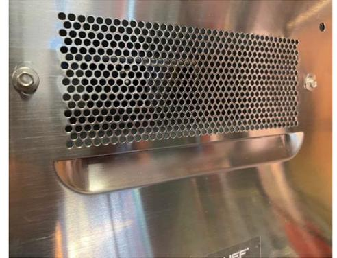
Air from the cooling fan is forced across the cooling fins of the magnetron(s) and into the cooling duct, which then vents the warmed air out of the back of the oven.
