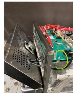
3. Disconnect the electrical connections; X523 on the IO board, the USB, ethernet and speaker loom connectors.
