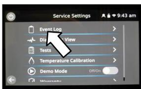
**12.** Check the "Event Log" for details of any logged appliance errors. Refer to the fault-finding section 5.3 to reference any errors logged.
