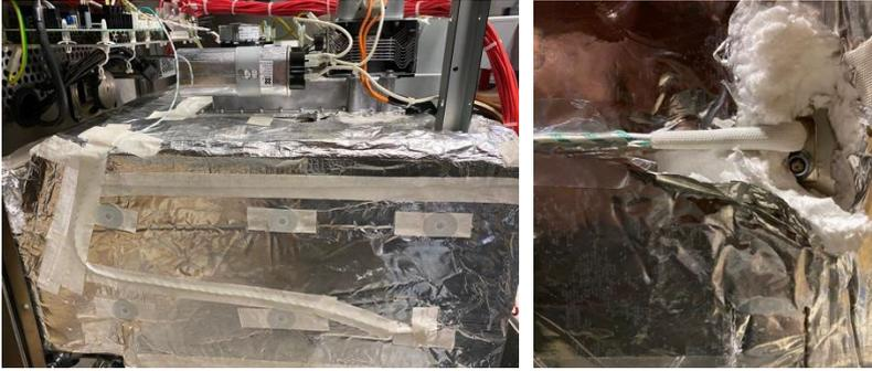
Cavity temperature measuring is done by a temperature sensor (thermocouple) connected to the IO Board.
