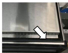
**6.** Check the door seal, ensuring that it is intact, not hanging loose or have any sections broken away or cracked. Replace if required and allow silicone to cure.
