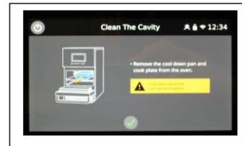
4. Once the cooling process is complete, remove the cook plate and pan of water if used. Then follow the screen instructions - the oven is now ready for cleaning.
