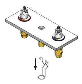
Step 2: Place hanger on body. Add center flange nut to top of compression nut.
