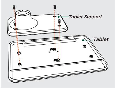
Rotate the Tablet Support mount from "R" to "L" and fasten it to the underside of the Tablet using the four Screws.
