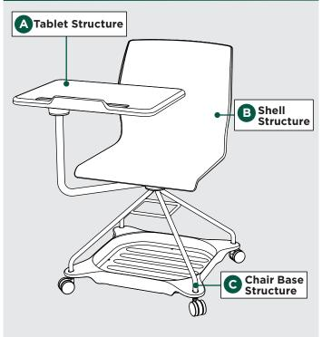
Face Shell Structure B downward, and place it on a flat surface.
