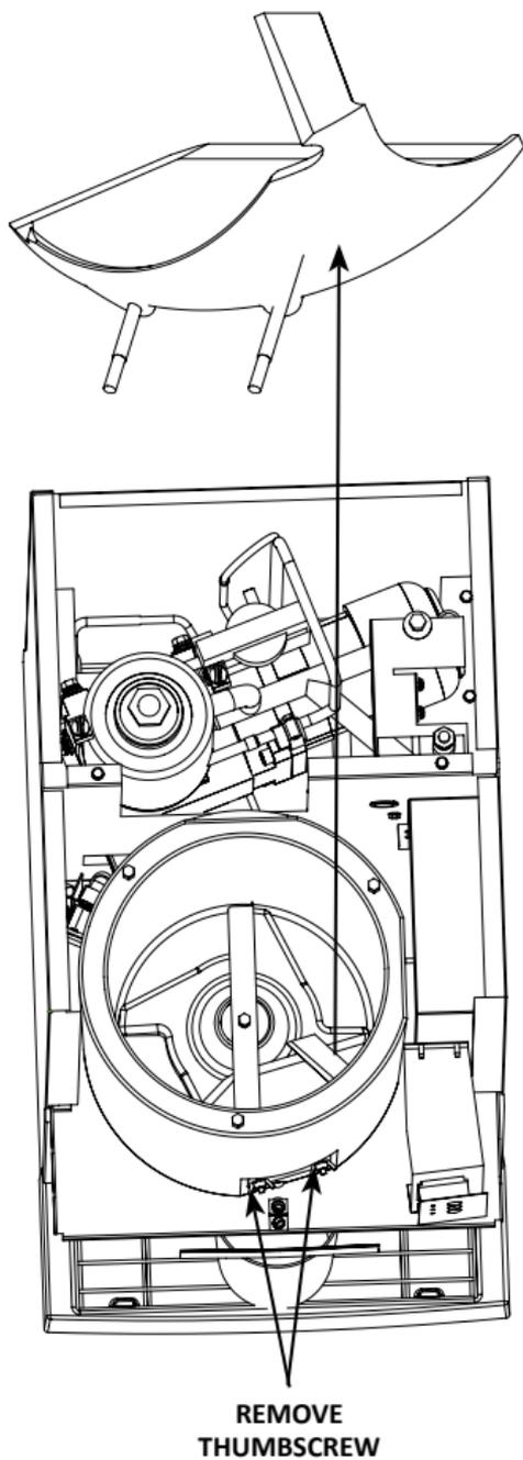
19. Remove ice dispensing wheel by lifting straight out.
