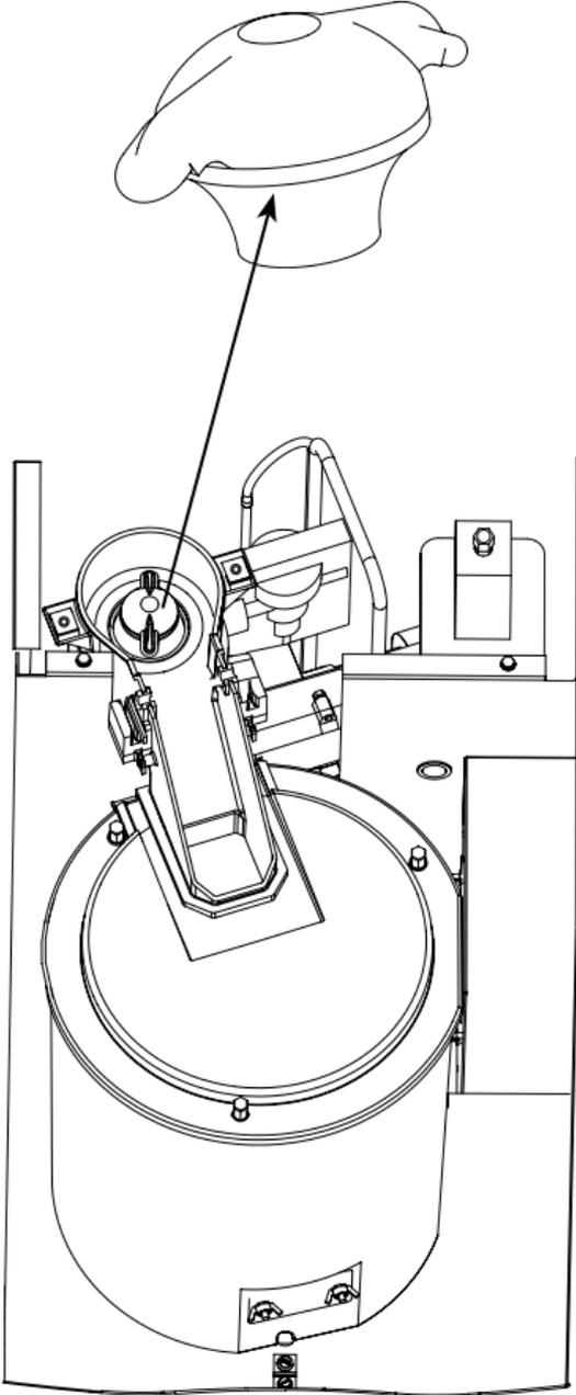
12. Loosen ice chute hose clamp.
