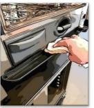
Clean out the two drip trays, wiping away from the drain holes
