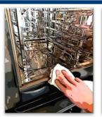
Wipe the rubber door gasket on door frame with a soft damp cloth
