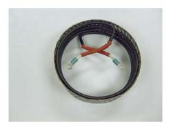
Step 7 – screen assembly removed from spinning head.
