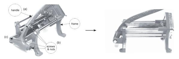
2. Connect **push block** in the center of **frame** ,and screw in firmly to frame.
