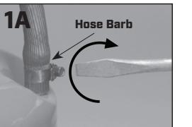
Make sure hose is pushed all the way to the tank. Make sure hose clamp is tight and below the hose barb. Turn clockwise with a screwdriver to tighten.
