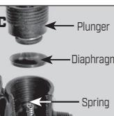
Remove plunger, diaphragm and spring. Wash diaphragm with mild detergent. Reassemble: Hold shut-off upright as shown, place spring in hole, place diaphragm on top of spring. Reassemble plunger and tighten.
