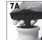
Turn handle clockwise to tighten. Push handle down, turn 1/4 turn clockwise to lock. Begin spraying.
