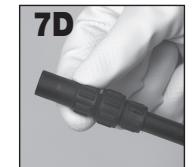
Adjust spray pattern by turning nozzle cap. Do not turn cap more than 2 turns or cap may come off allowing spray material to spray back on you.
