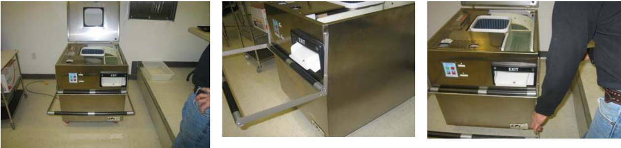
2. Using the appropriate screwdriver, remove the basket holder from the unit.
