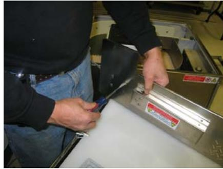
5. Using the appropriate screwdriver, remove the clips that secure the electric cord to the unit.
