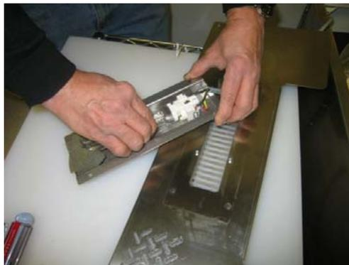
7. Leaving the sponge in place in the UV-C cavity, gently remove the lamp from the ballast and replace with the new UV-C lamp.
