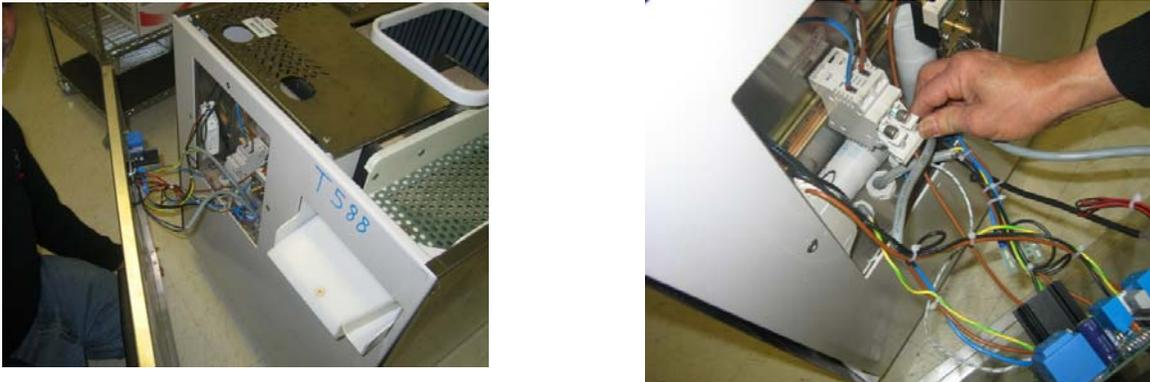
4. **Gently** remove the panel from the unit. Ensure that the fuses have blown and replace them.
