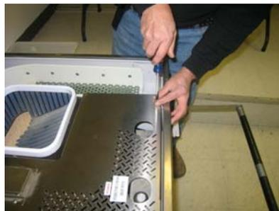
4. Remove the stainless steel tank cover of the unit by removing the three panel screws.
