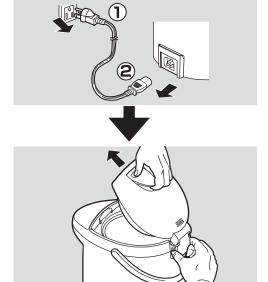
Hold the product with both hands and dispose water where indicated "EMPTY FROM HERE" on the wall of the Inner Container.
