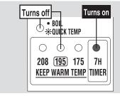
The TIMER light, the BOIL/QUICK TEMP light and the KEEP WARM light turn on at the same time for 2 seconds.
