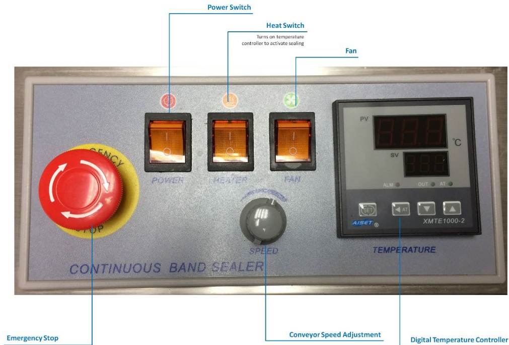
Figure 9. Control Panel of CBS-880
