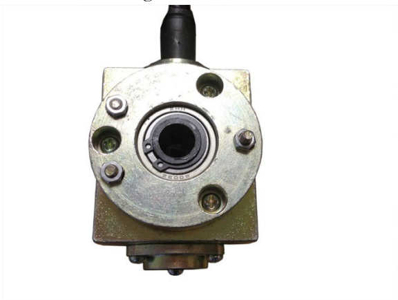
Figure 25. Remove the three screws and nuts on the umbrella gear.
