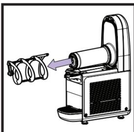
2. Remove the outer magnetic rotor assembly. The assembly is secured to the evaporator by a magnet and may need sufficient force to break the magnetic field.
