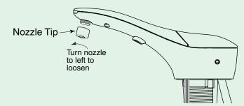
DO NOT use abrasive or chemical cleaners (including chlorine bleach) to clean Spout, as it may dull the luster and attack the chrome-plated exterior. Use ONLY mild soap and water, then wipe dry with clean cloth. While cleaning the bathroom counter top, protect the Spout from any splattering of cleaner. Acids and cleaning fluids will discolor or remove chrome plating.
