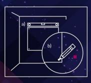
1) Place your sign on the wall (optional: Use leveler). With the pencil, mark the center of the holes where the screws will go.
