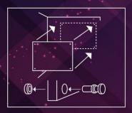
5) Align your sign with the holes and screw the caps with the rubber washer through the sign into the barrel.
