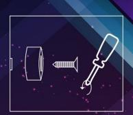
4) Take your standoffs and unscrew the cap from the barrel. Secure the barrel on the wall using a screwdriver and the screws included. \*Make sure it is tightly secured as this will be holding your sign.
