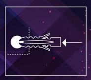
3) Insert your anchors in the holes. Hammer the anchor lightly until it is flush with the wall.
