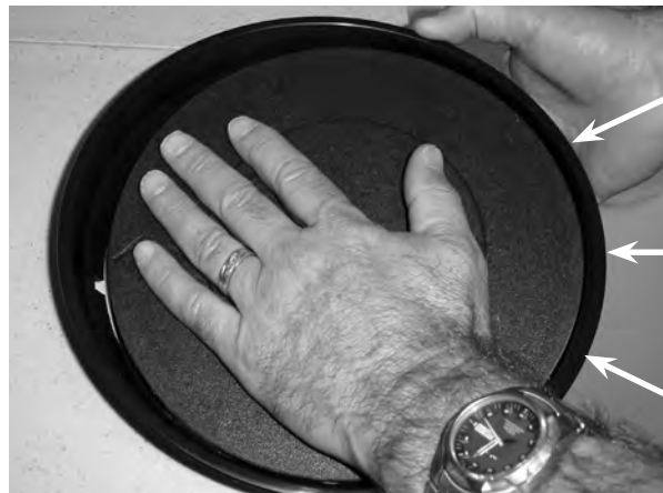
Step 4: Place the Base Rim with the Base Pellet on the edge of a table. Holding the Base Pellet down with your left hand, pull the Base Rim out with your right hand in three places as shown above, until the Base Pellet snaps securely into place.
