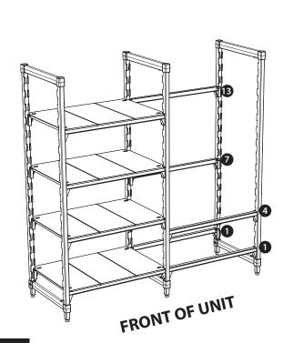
• = Traverse installation position on dovetails
