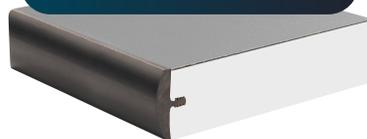
**T-Mold Edge** is characterized by a T-shaped molding that is inserted into a groove along the edge of the tabletop. The T-Mold is made of a durable and flexible material, that is able to withstand wear and tear and is stapled to the underside of the tabletop for added resilience.
