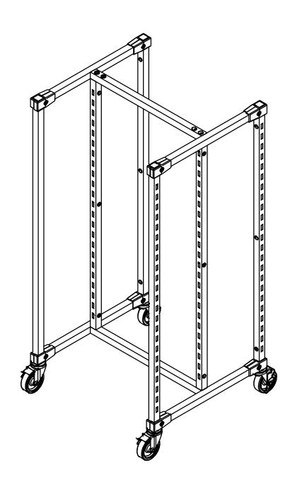
Step 1: Connect the two side Before starting, identify which frames to the center panel. side is the top of theframes. The top of the frame has the Step 2: Attach casters. first slot 3-1/4" from the top. The bottom has the first slot 5-3/8" from the bottom. ATTACH **CASTERS**
