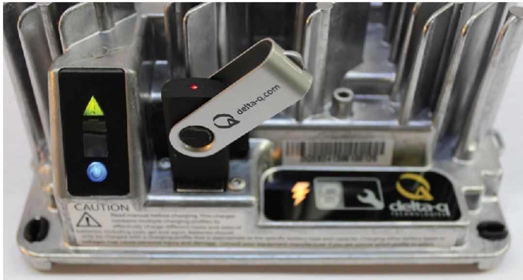
Figure 5, Insert the USB flash drive to begin the charge data download process. This step can be completed using the same USB flash drive programmed to update the charger's software. The process is complete when the USB indicator is solid green, and no longer flashing.
