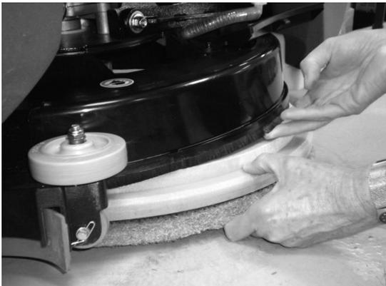
6. Check that release lever/plate is completely closed and pad/brush is securely attached.
