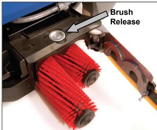
4. Slide new brushes into receptacle at far side of deck, lift upward and snap into position. Ensure brushes are secure.
