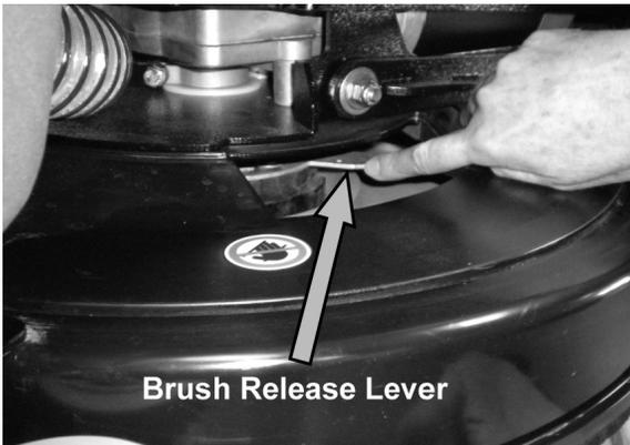
4. Remove brush/pad from holder and replace with new brush/pad.
