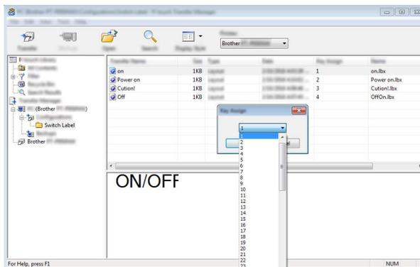
The data registered with keys 1 to 28 (1) of the one-touch panel is determined by the key number.
