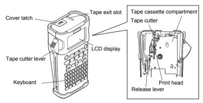
When shipped from the factory, the LCD display is covered with a protective sheet to prevent damage. Remove this sheet before using the P-touch.
