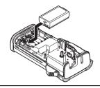
Confirm that the hooks on the edge of the rear cover are inserted correctly, and then reattach the cover
