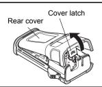
Insert the rechargeable Li-ion battery into the battery compartment.
