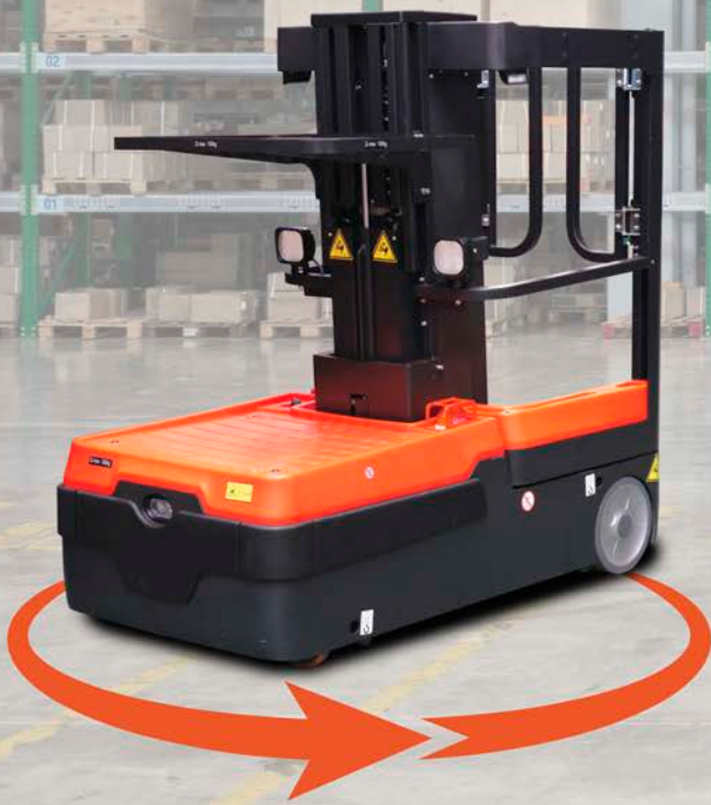
360° Zero-turning radius of 51.2 inches
