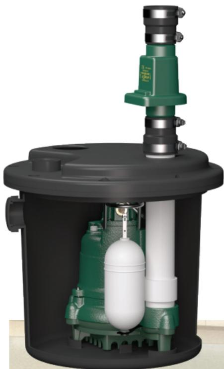
Designed for applications where gravity flow is not possible including laundry tray, wet bar sink, lavatory, air conditioning condensate, and dehumidifier. Can also be used in conjunction with dishwashers or garbage disposals and conveniently fits inside cabinets for a clean look.
