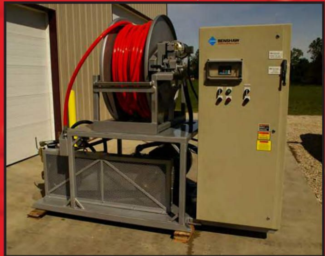
11 gpm, 2000 PSI Hot Water skid machine for Los Angeles Water District.
