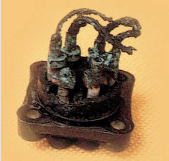
Photo showing acid attack on the compressor's terminal wires
