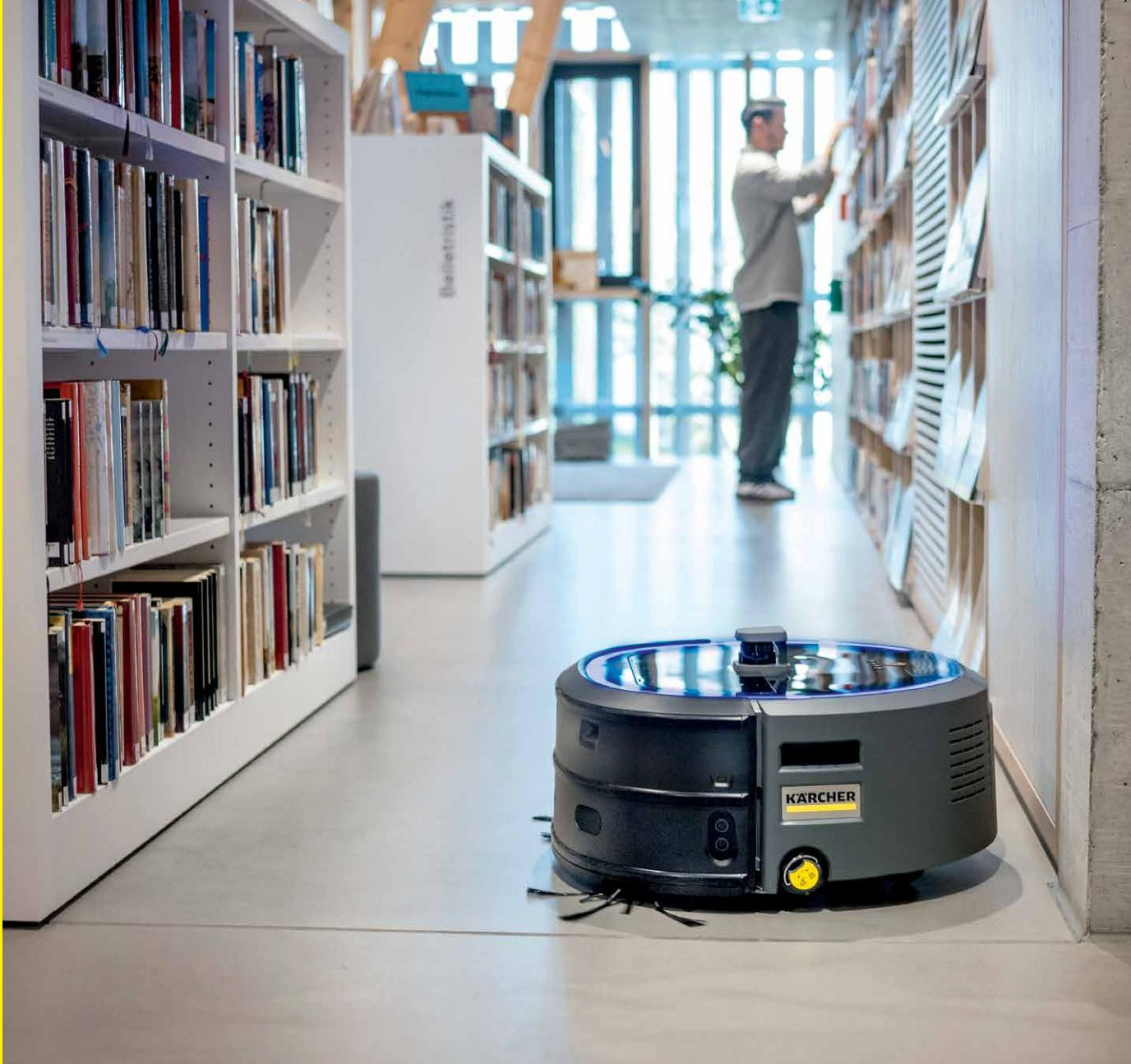
**Intelligent navigation.** Areas that experience heavy foot traffic tend to get dirtier. With the KIRA Robots app, you can edit the cleaning maps later on and instruct the vacuum cleaner to clean extremely dirty areas twice. The intelligent sensor system ensures precise cleaning in these specific areas, resulting in high cleaning quality.
