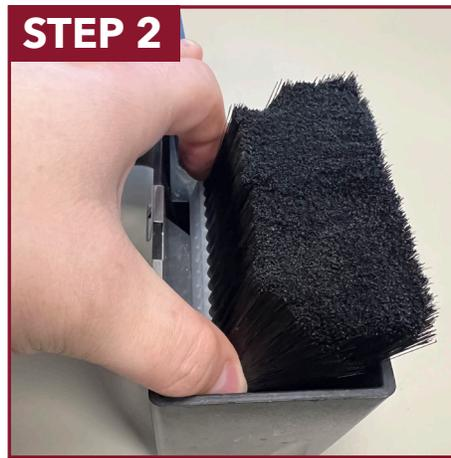
With equal pressure on both sides of the brush, push down on the brush base to slide the base of the brush between the water tank and retaining clip.
