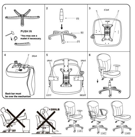
Insert and loosely tighten all screws. When assembly is completed, fully tighten all screws before using. This chair is only intended for sitting. Any other use will void the warranty.
