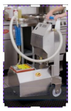
With the pump ON, ensure that the Wand nozzle is directing the oil into the fryer vat. While holding the blue handle on the top of The BOSS, rocking back and forth should free up the air lock and start the flow of oil.
