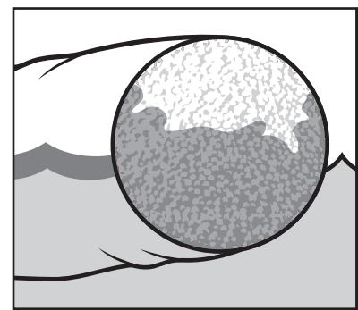
As the spill is absorbed, the boom floats lower in the water. Oil is now exposed to fresh absorbent.
