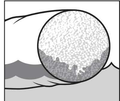
Put in spill on water. Boom begins to absorb as soon as it's in place. No water soaks in – only petroleum products.
