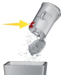
2 Hold over trash can and press the dirt cup release to empty.
