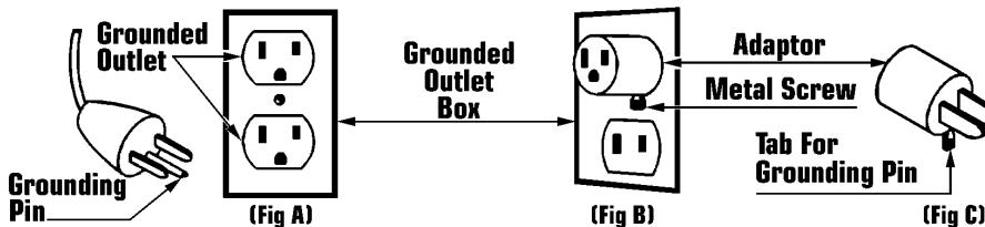
This electric equipment is for use on a nominal 120 volt circuit, and has a grounded plug that looks like the plug illustrated in (Fig A). A temporary adaptor that looks like the adaptor illustrated in (Fig B & C) may be used to connect this plug to a 2-pole receptacle as shown in (Fig B) if a properly grounded outlet is not available.
