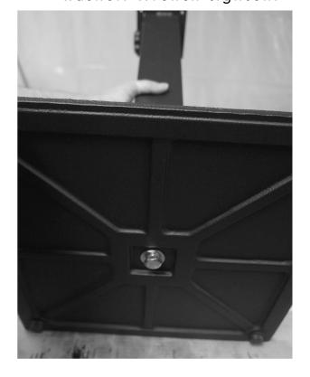
3. Position the spider plate to the top of the column. Attach with the 4 small screws.
