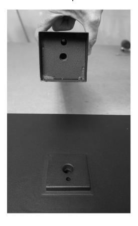
2. Fasten the base plate to the column with the bolt, the flat washer and then the lock washer. Wrench tighten.
